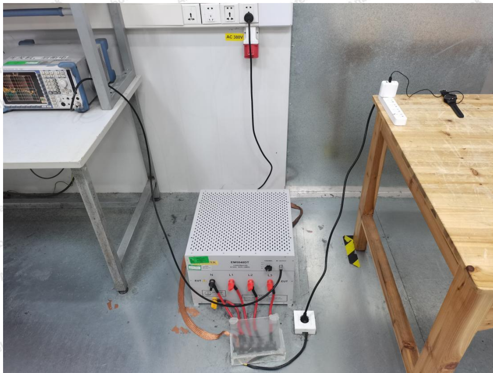
Photo of Conducted Emission Measurement
