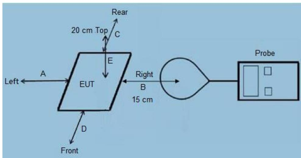
The measurement probe was placed at test distance (15 cm from all sides and 20 cm from the top) which is between the edge of the charger and the geometric center of probe.
