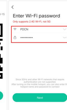
(7) Enter WiFi password The device only supports 2.4G network
