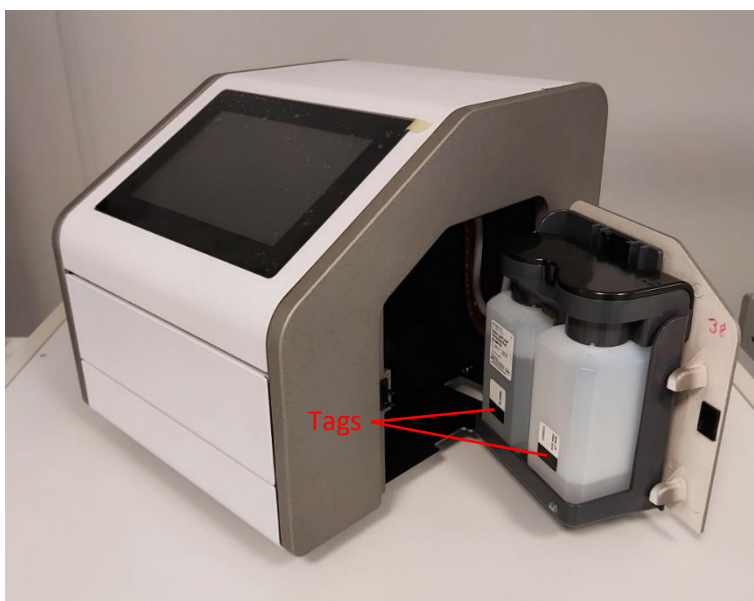
Fig. 2 - opened fluid/liquid bottles compartment with partitioning fluid and waste bottle
