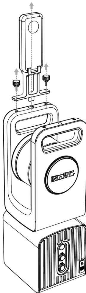
Figure 3-2.4 Disassembly diagram of HD TLS360 system camera
