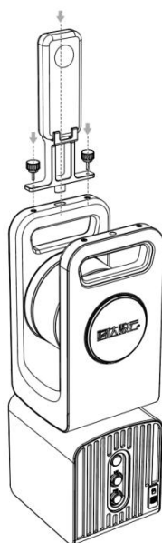
Figure 3-2.3 Installation diagram of HD TLS360 system camera
