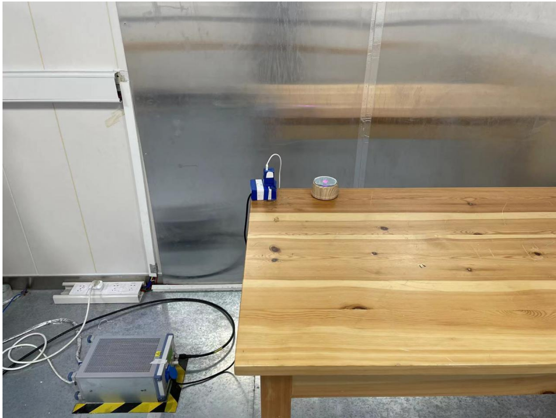
Conducted emission test setup
