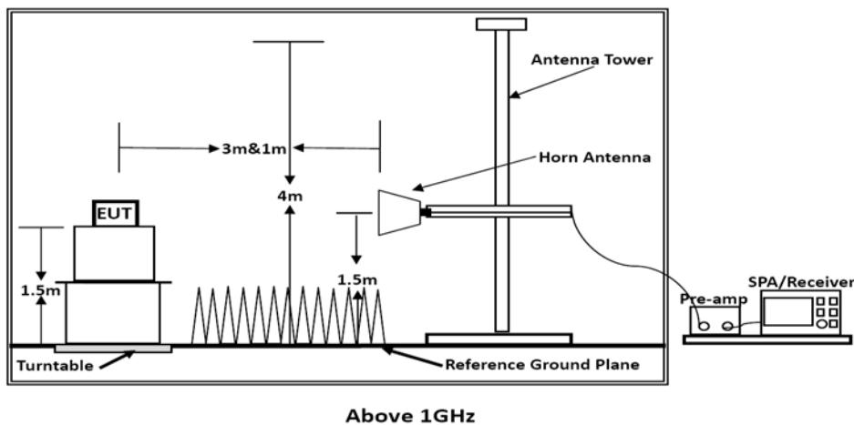
Above 18 GHz shall be extrapolated to the specified distance using an extrapolation factor of 20 dB/decade from 3m to 1m.
