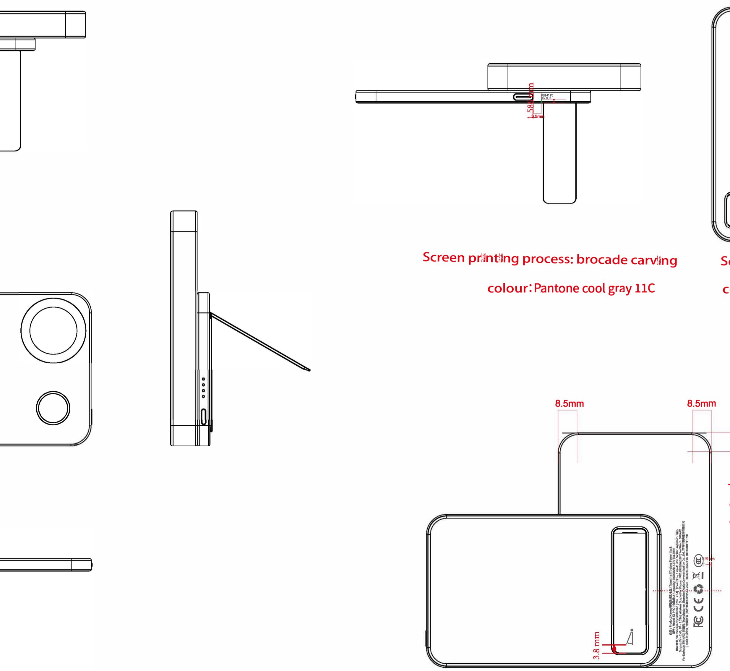
Requirements: 0.65glas ±0.05explosion-proof film the total thickness of the finished product is below 0.75 without baking glue
