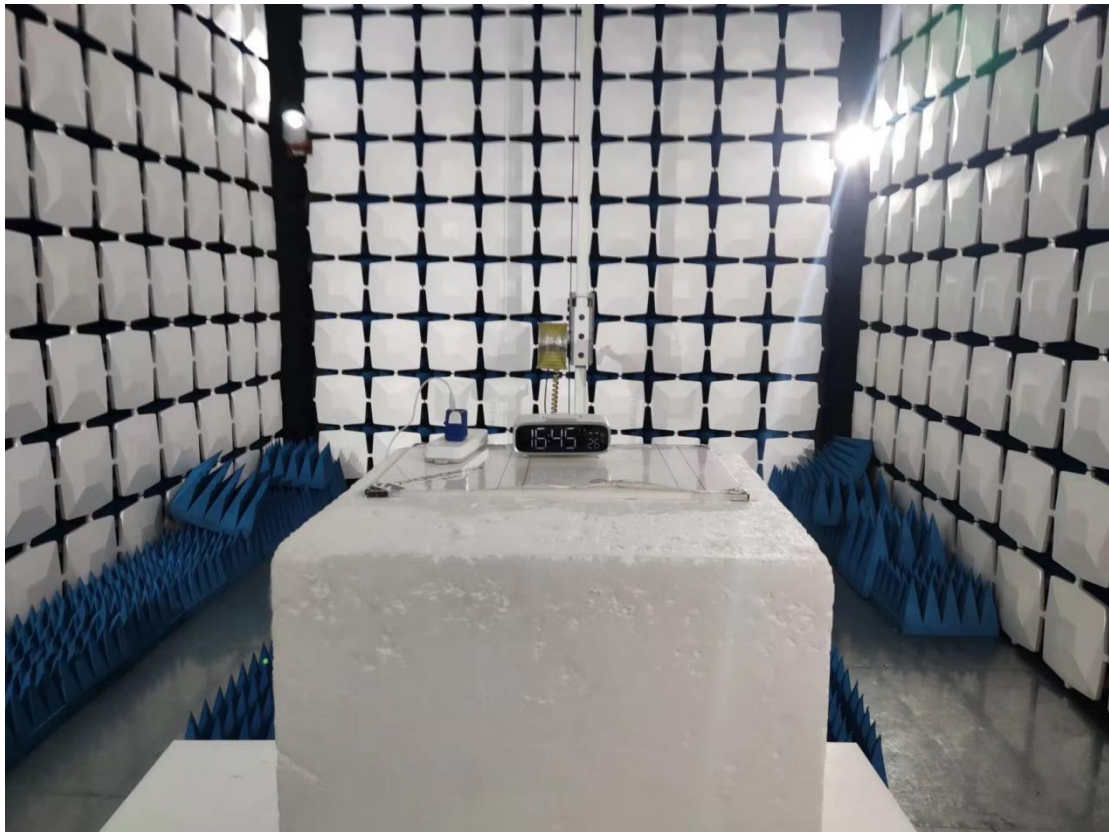
Above 1GHz for radiated emission test setup
