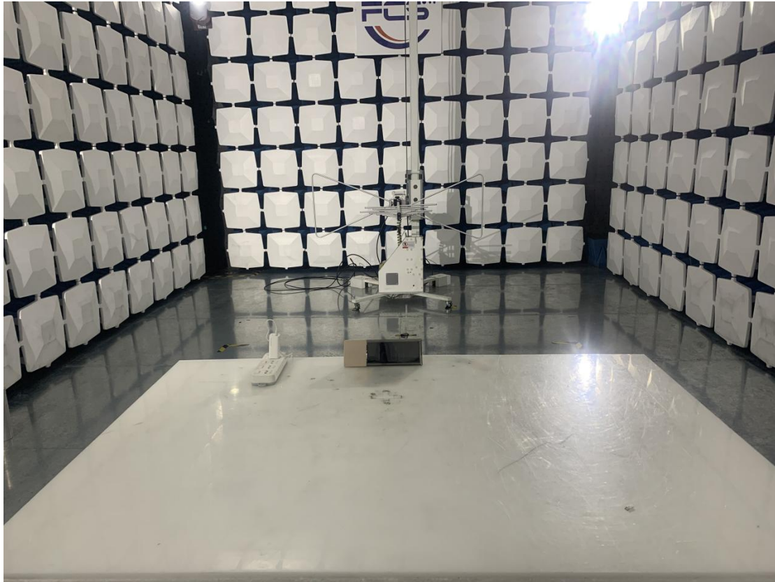
Above 1GHz for radiated emission test setup
