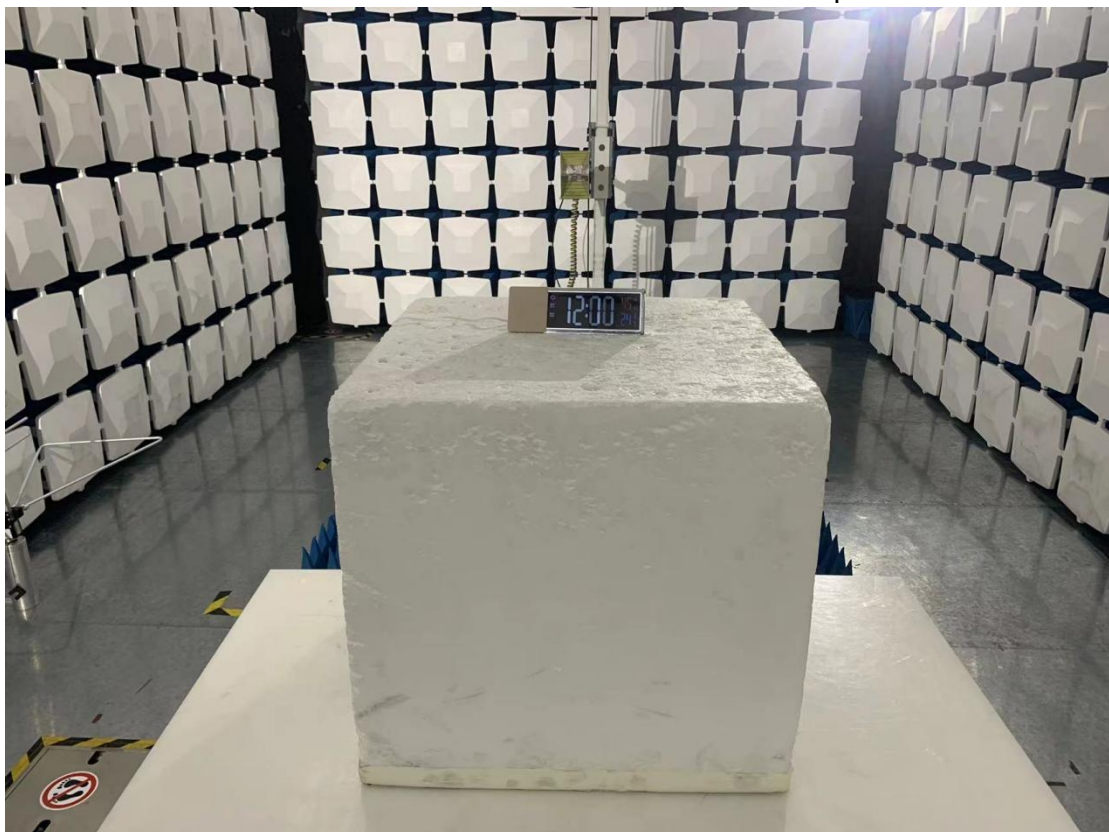
Above 1GHz for radiated emission test setup
