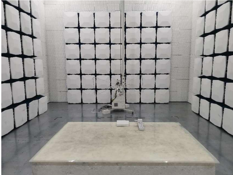
RADIATED EMISSION MEASUREMENT (below 1G)
