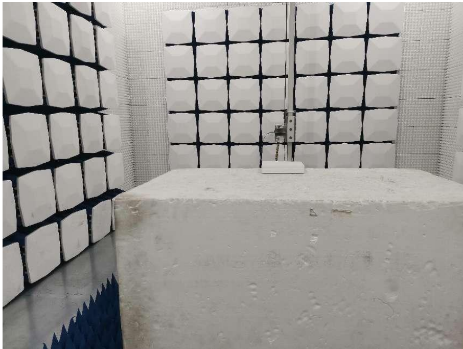
RADIATED EMISSION MEASUREMENT (Above 1G)
