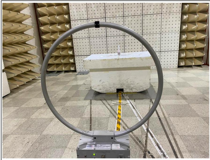
**3. Photo of Radiated Spurious Emission Test (30 MHz ~ 1 000 MHz)**
