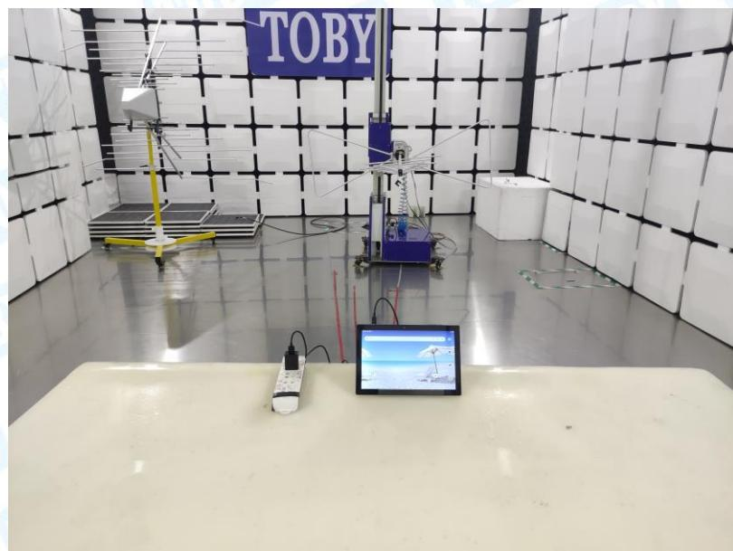
**Photo of Setup for Conducted Emission**
