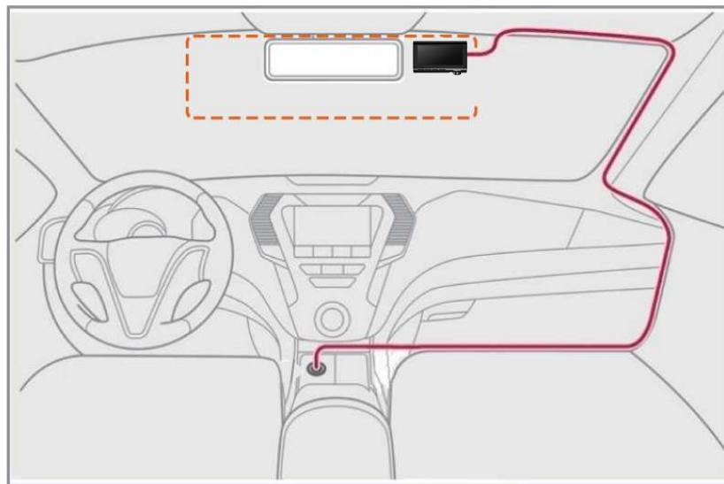
2. Clean the spot on your windshield where you would like to mount the camera and confirm the placement. We recommend to install the camera near the rear view mirror of driver opposite side.
