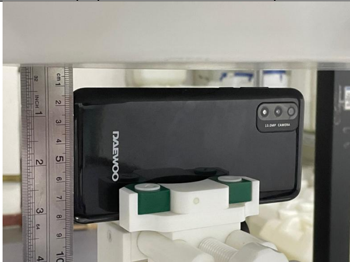
Bottom Side (Separation distance of 10mm)
