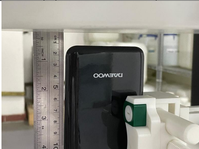
Bottom Side (Separation distance of 10mm)
