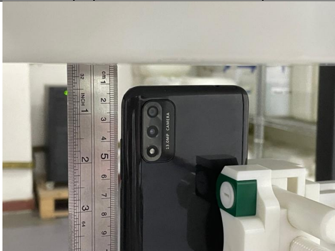
Top Side (Separation distance of 10mm)
