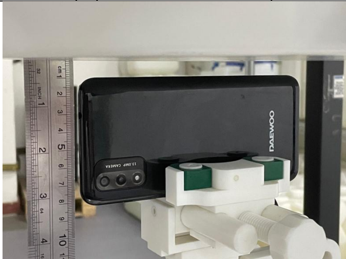
Top Side (Separation distance of 10mm)
