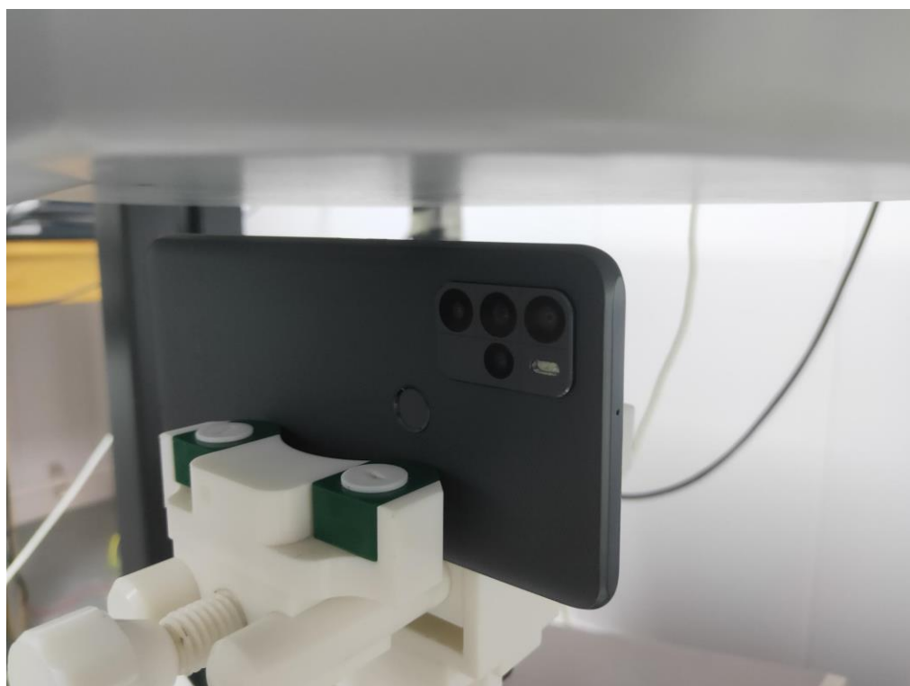
10mm body-worn Right Side Setup Photo (hotspot)
