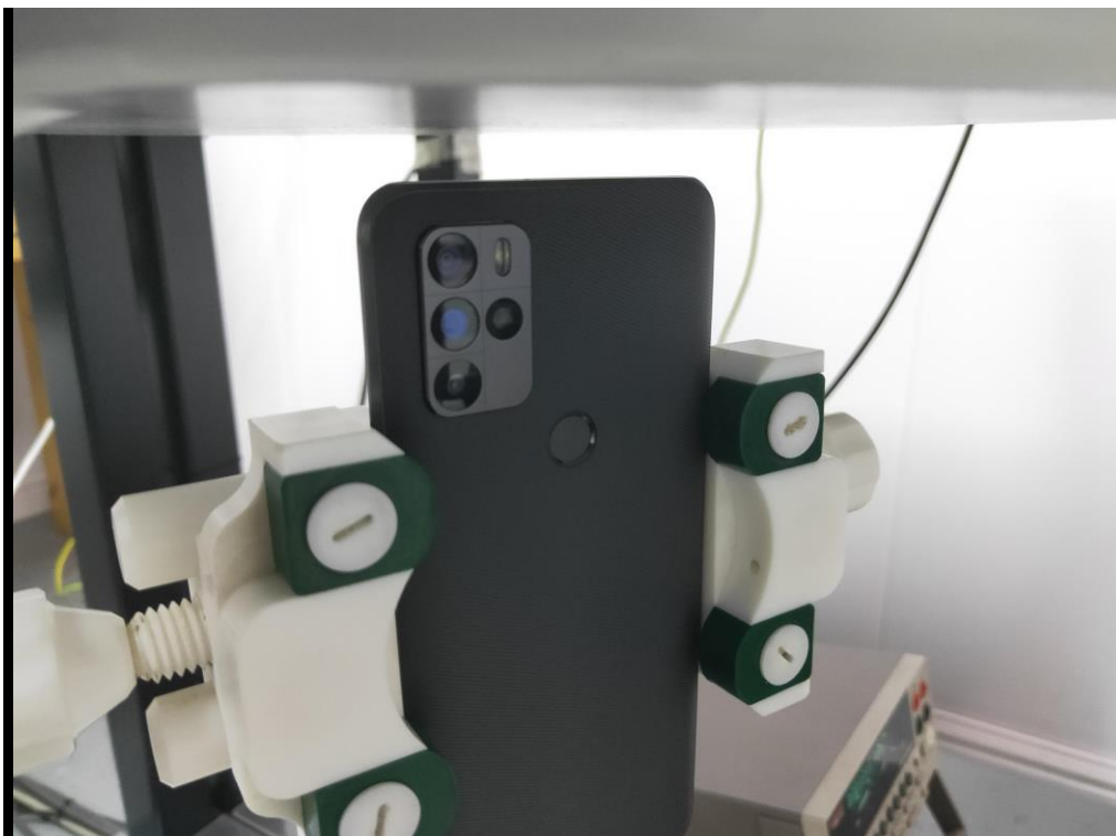
10mm body-worn Top Side Setup Photo (hotspot)
