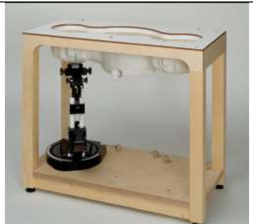
Fig. 8.7 Photo of SAM Twin Phantom
