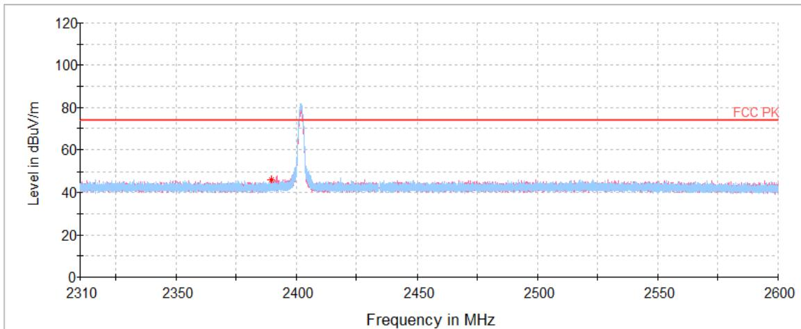
**Horizontal/Vertical for 1 GHz ~ 3.5 GHz**
