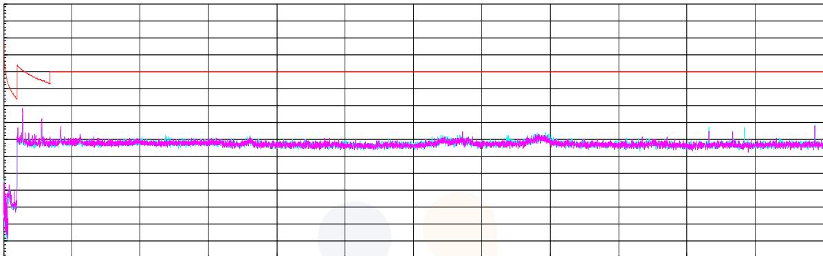
**Test results (Below 1 000 MHz) – Worst case: GFSK\_2 480 MHz**
