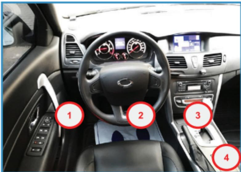
When the car is turned off, attach the terminal to OBD socket shown above, and start the car (red LED light is up when installed normally).
