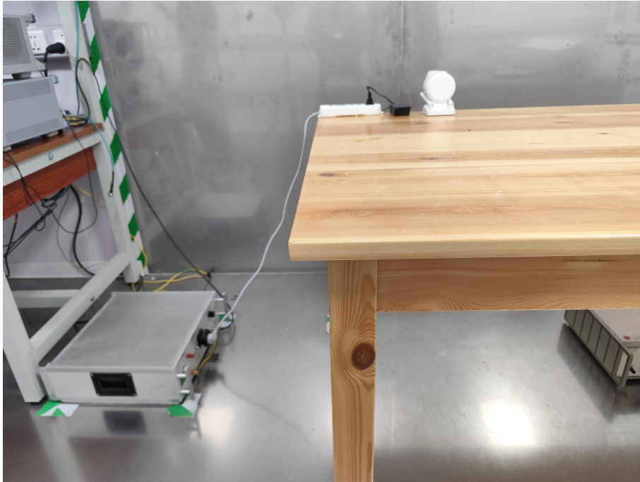
Conducted Emission at AC power line
