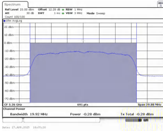
Conducted AVG output power IEEE 802.11n_20_Channel 52_Antenna 0
