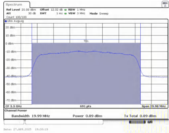
Conducted AVG output power IEEE 802.11ac_20_Channel 100_Antenna 0
