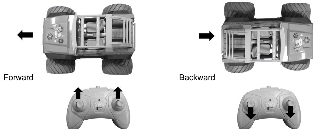
**1. Forward** Push the left and right control levers upward, the RC car moves forward
