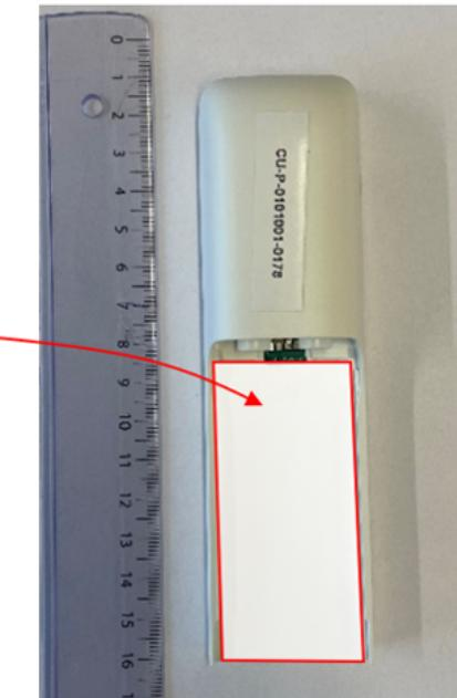
The label is placed on the CU01 clearly visible by the user. The label will be covered when a Cartridge is attached. The cartridge is a replaceable drug compartment (refill), that is attached and removed by the user.
