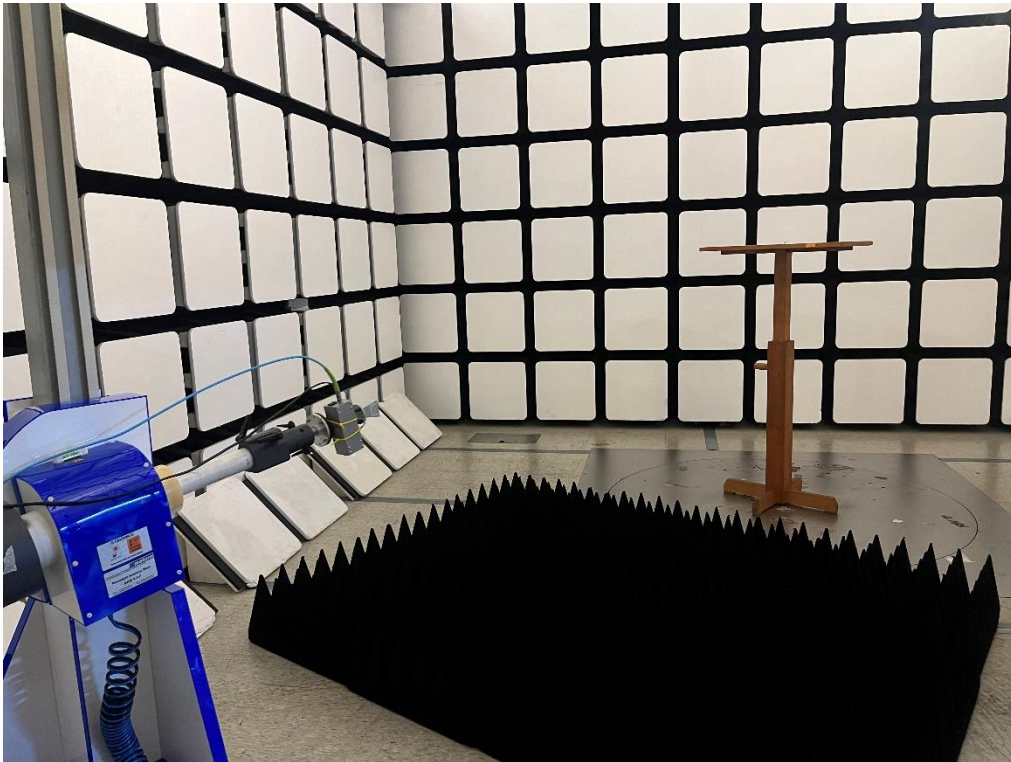
Photo 3: Measurement above 1 GHz (18 GHz to 40 GHz)
