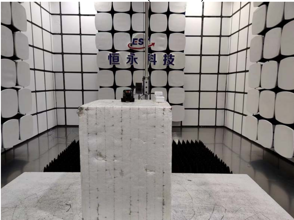
Radiated Test (Above 1GHz)
