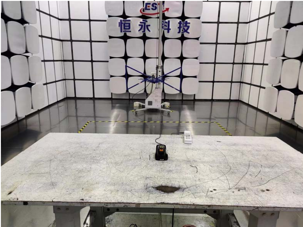
Radiated Test (Below 1GHz)
