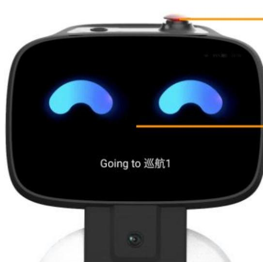
In case of emergency, press the emergency stop button and the robot stops immediately.
