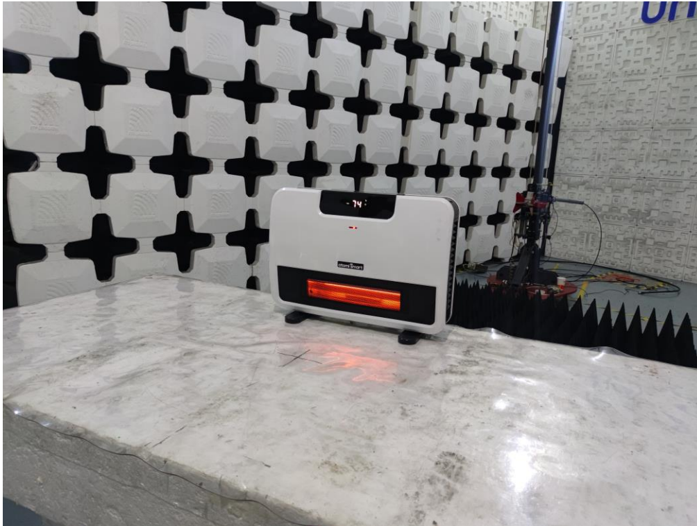
Radiated emission Test Setup-2 (Above 1 GHz)
