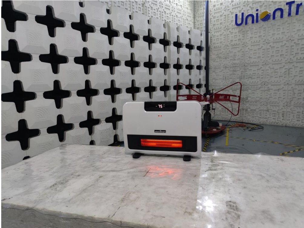
Radiated emission Test Setup-1 (30 MHz~1 GHz)
