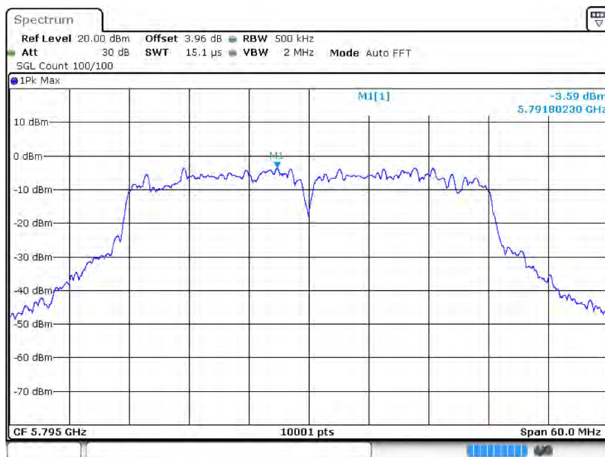
PSD ac40 5795MHz Ant2
