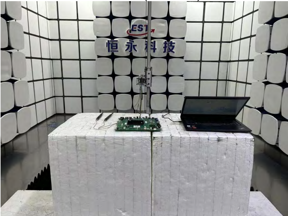
Radiated Test (Above 1GHz)
