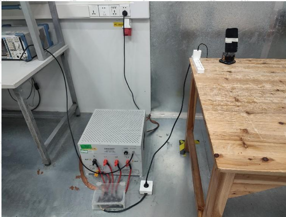
Photo of Conducted Emission Measurement
