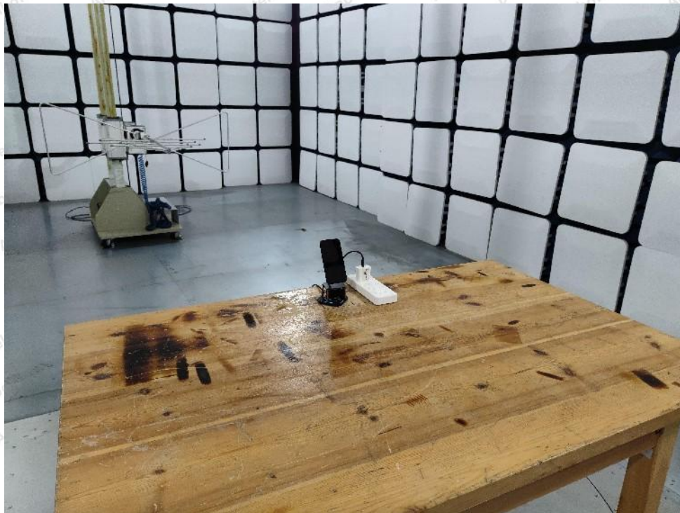
Photo of Radiation Emission Test
