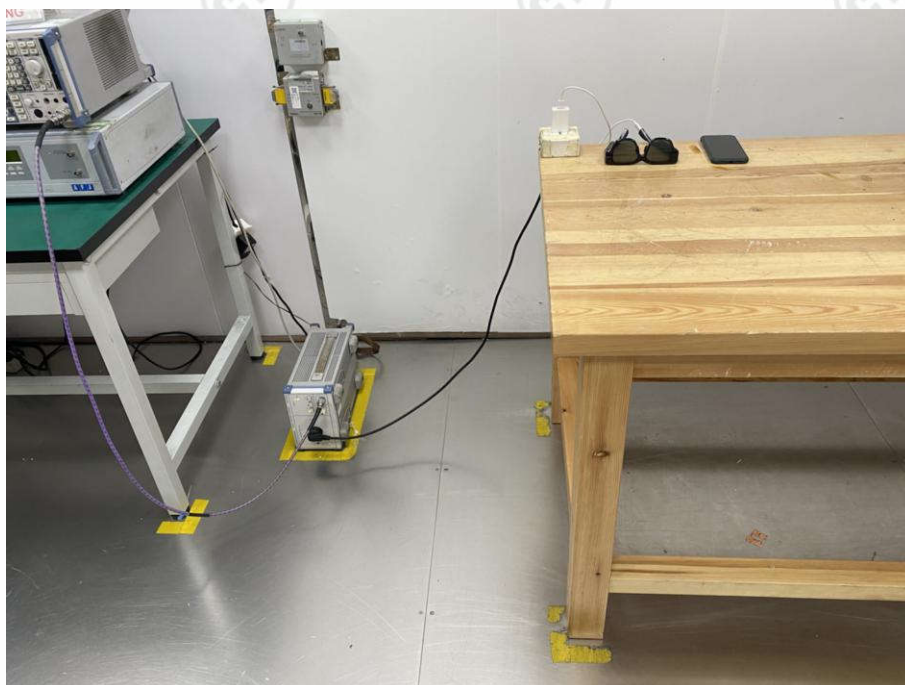
Conducted Emissions Test Setup
