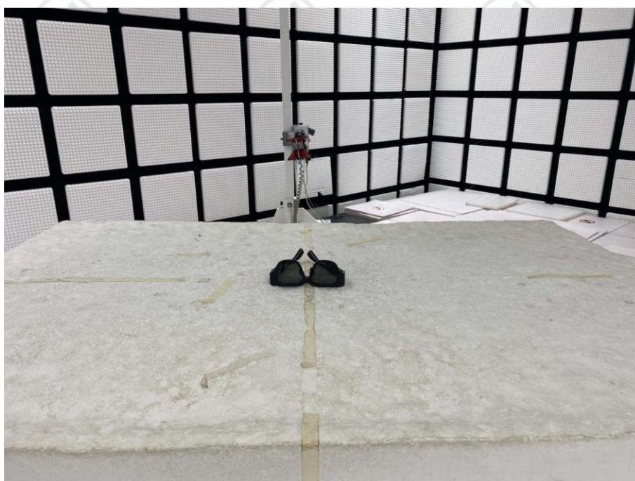
Radiated spurious emission Test Setup-2(Above 1GHz)
