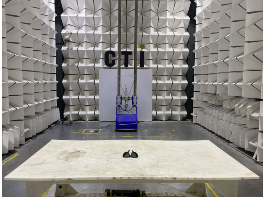
Radiated spurious emission Test Setup-1(Below 1GHz)
