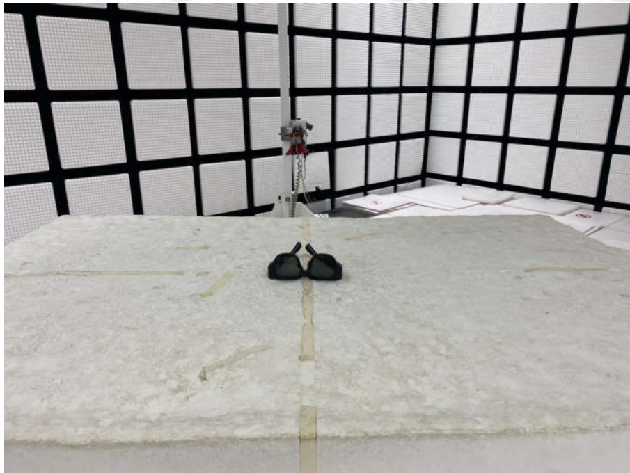
Radiated spurious emission Test Setup-2(Above 1GHz)
