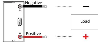
4.2.2 Using in Series or Parallel (A maximum of 16 batteries can be connected in parallel and 4 batteries can be connected in series. Note: It is forbidden to use series and parallel simultaneously)
