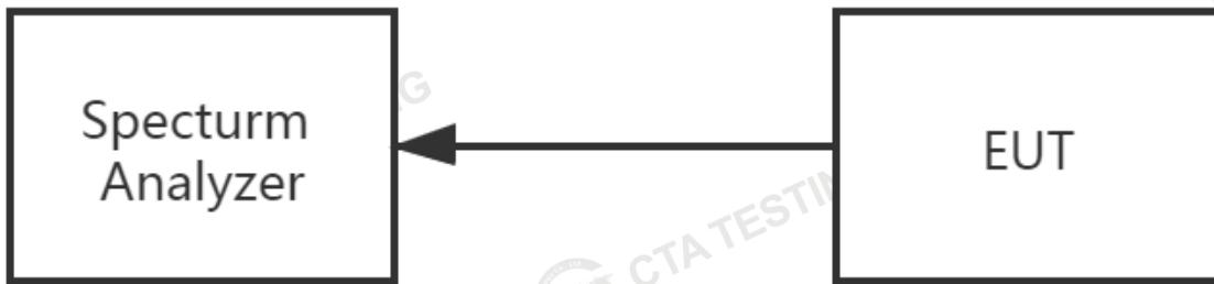
The EUT is connected to the Spectrum Analyzer; the RF load attached to the EUT antenna terminal is 50 Ohm; the path loss as the factor is calibrated to correct the reading. Make the measurement with the spectrum analyzer's resolution bandwidth(RBW) = 100 kHz. In order to make an accurate measurement, set the span greater than RBW.
