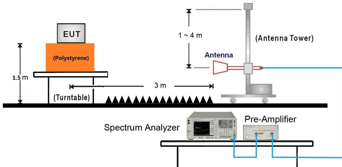
18GHz ~25GHz Test Setup:
