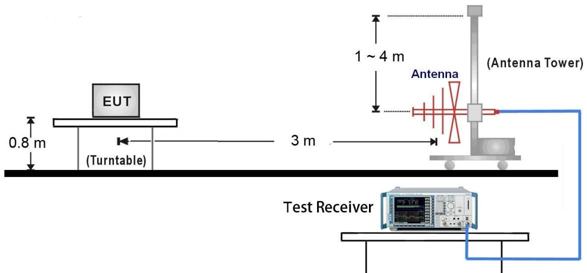
1GHz ~ 18GHz Test Setup:
