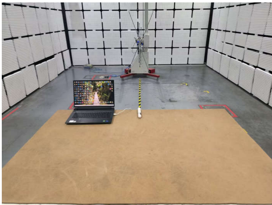
Radiated spurious emission Test Setup-1(Below 1GHz)
