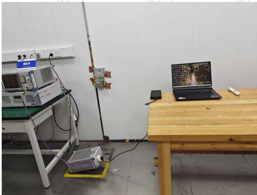
Conducted Emissions Test Setup
