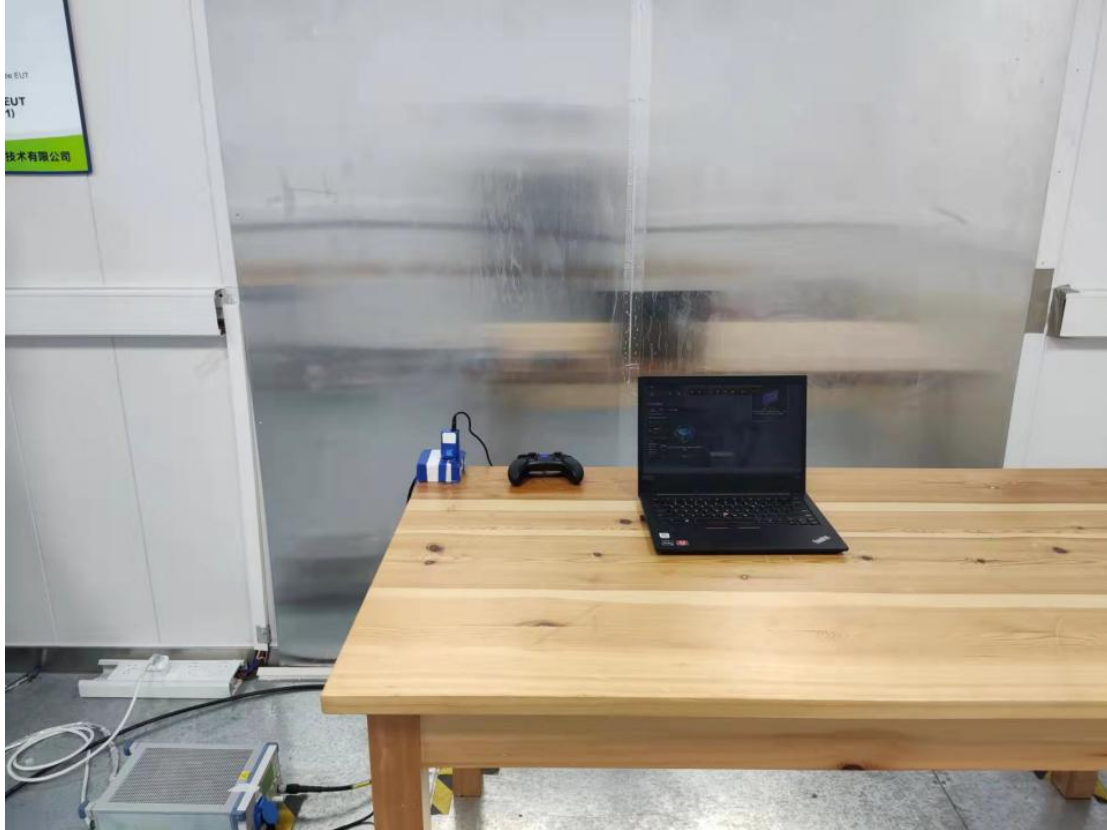
Conducted emission test setup
