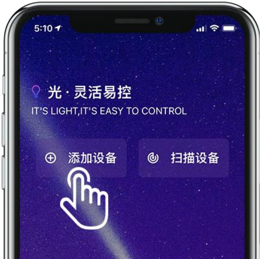
②Confirm that the current mobile phone is connected to WiFi, the App will automatically fill in the WiFi connected to the current mobile phone, you need to manually enter the password, click the connect button (note: 5GHz WiFi is not supported)
