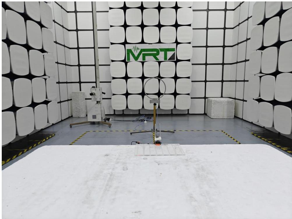
Description: Radiated Spurious Emissions Test Setup for 9kHz ~ 30MHz (Zoom Photo)
