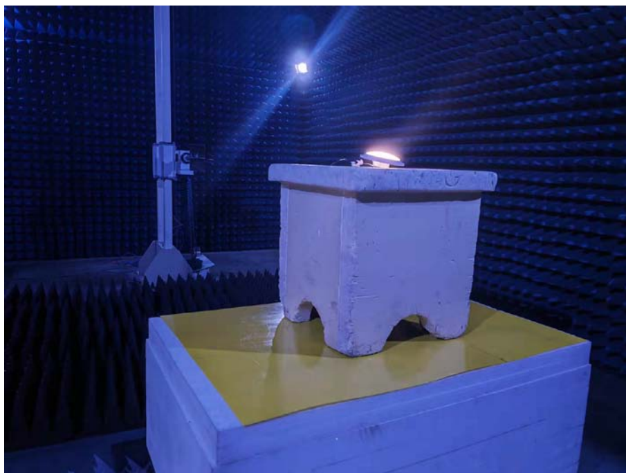
Photo of Radiated Emission Measurement Above 1GHz
