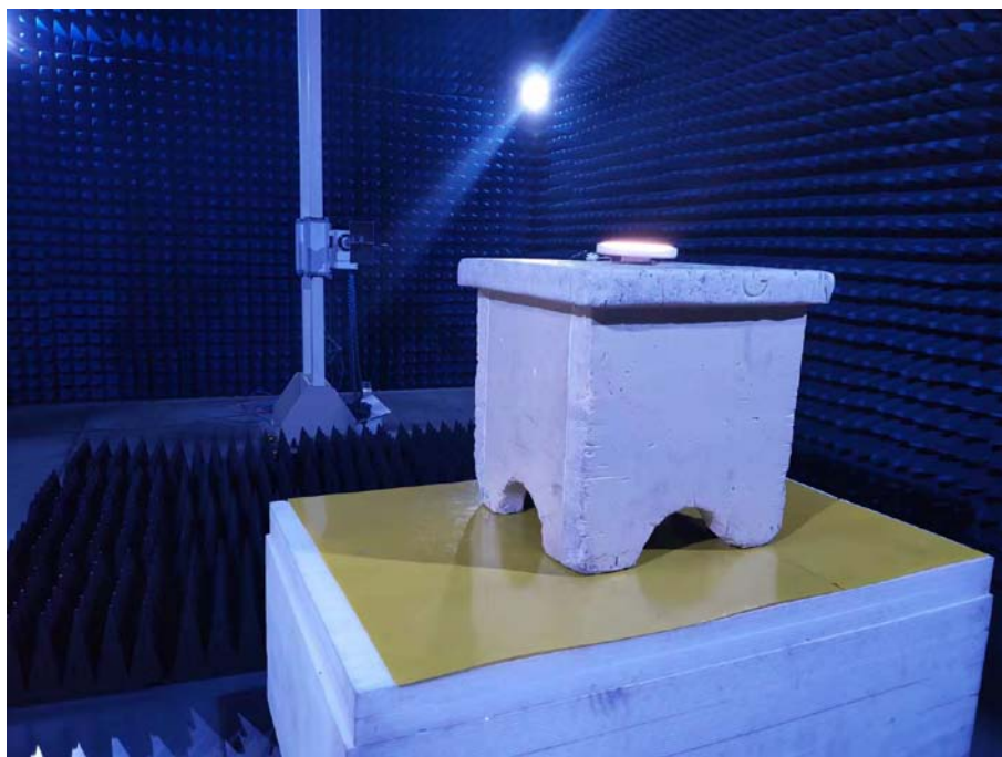
Photo of Radiated Emission Measurement Above 1GHz
