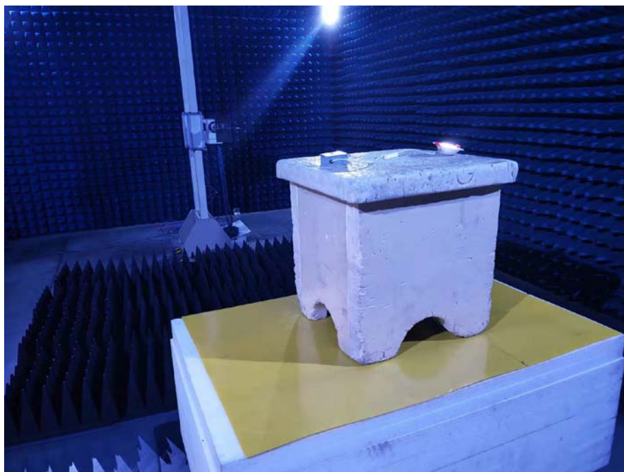
Photo of Radiated Emission Measurement Above 1GHz
