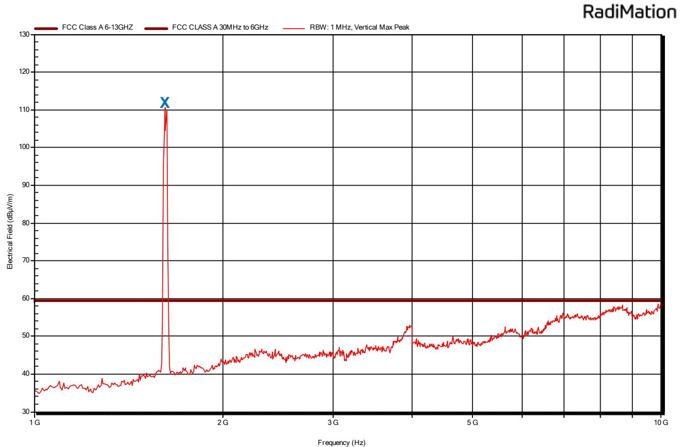
**Note:** X is related to the intentional radiating Iridium transmitter at 1626.5MHz and no measurement is required against the FCC Part 15b limit.
