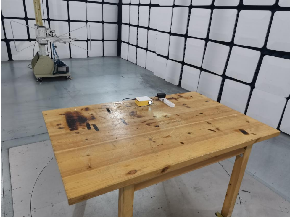
Photo of Radiation Emission Test
