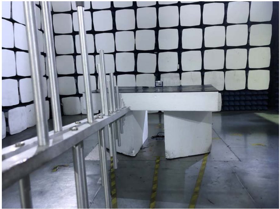
Radiation Emission Test Setup (30MHz to 1GHz)
