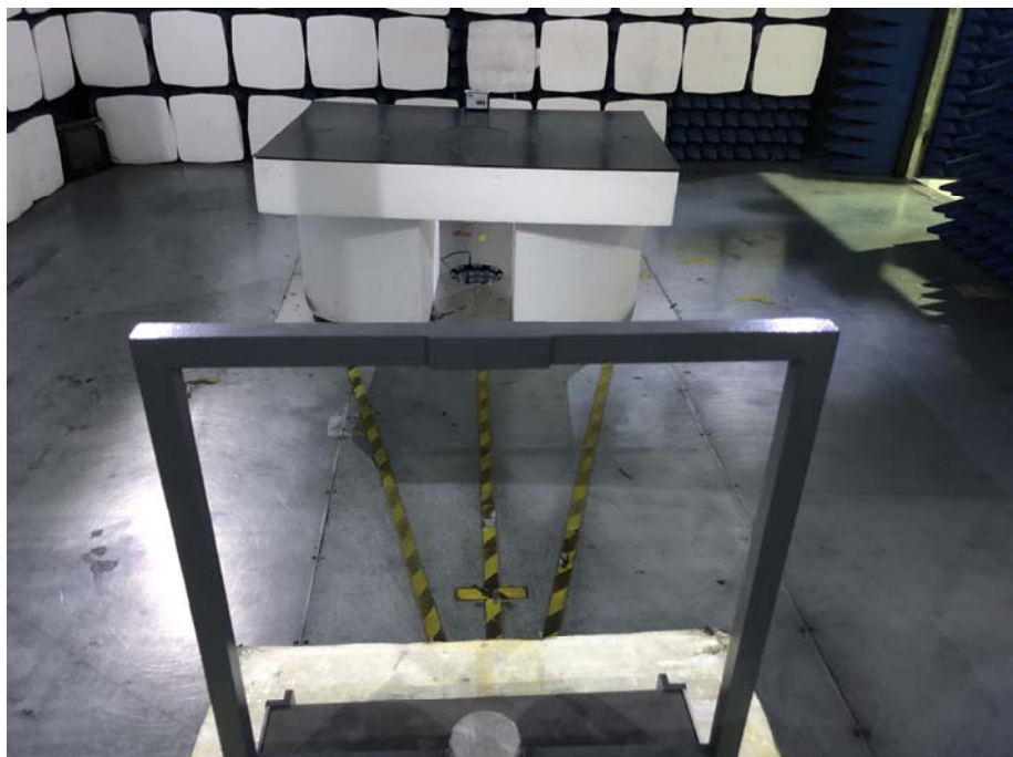
Radiation Emission Test Setup (Below 30MHz)
