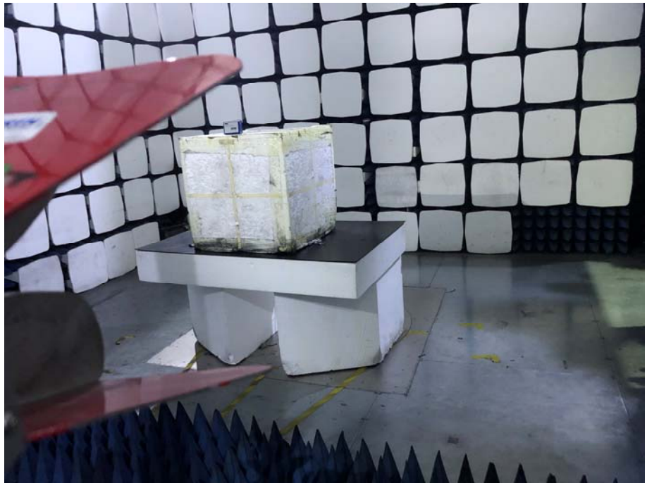
Radiation Emission Test Setup (1GHz to 18GHz)
