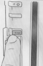
**Step 4:** Wait for a few seconds, the Player LED on the controller will stop flashing and light up when paring is complete. The Player LED indicates the player number of the controller currently in use.
