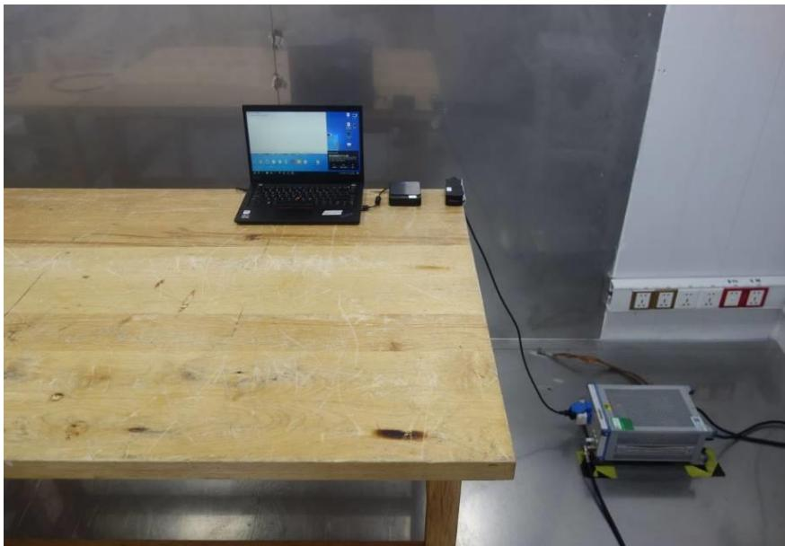
Radiated Emissions (9kHz-30MHz)
