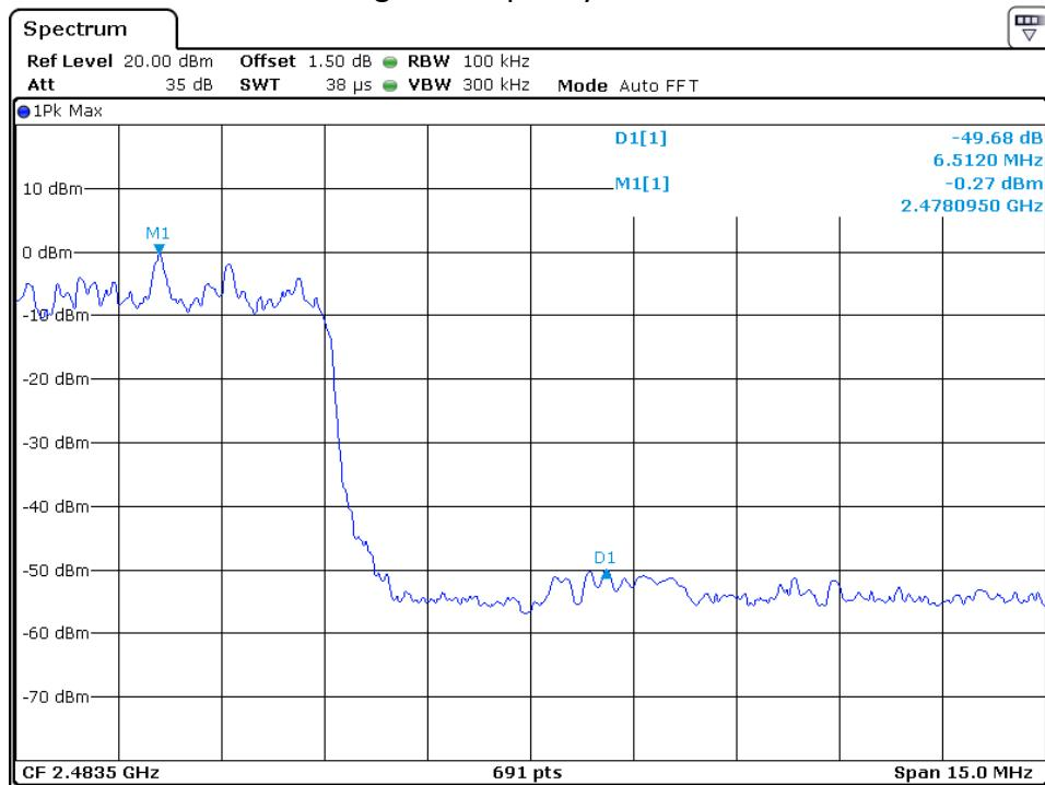
**4.9 Transmitter Spurious Emissions (Conducted)****Out of Band Conducted Spurious Emissions, FCC Rule 15.247(d):**
