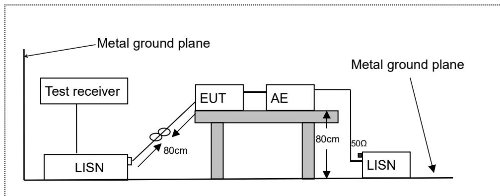
LISN: Line Impedance Stabilization Network
