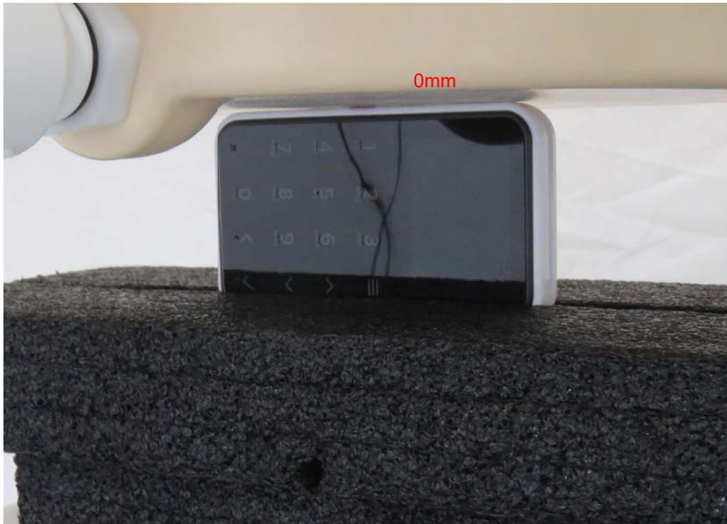
Picture 5: Left Edge, the distance from handset to the bottom of the Phantom is 0mm
