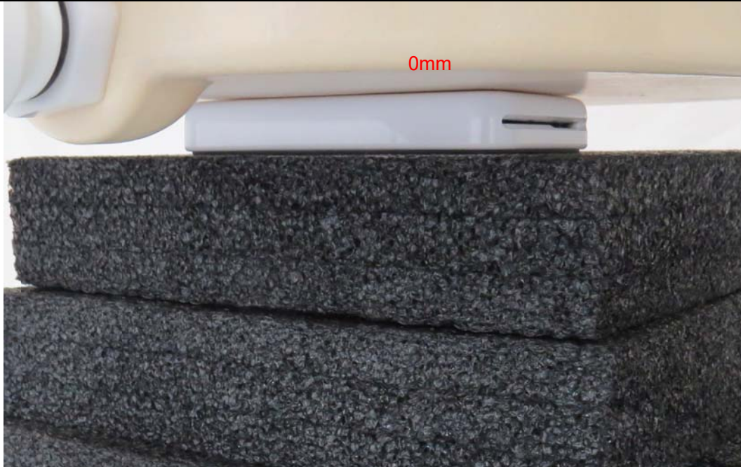
Picture 3: Back Side, the distance from handset to the bottom of the Phantom is 0mm
