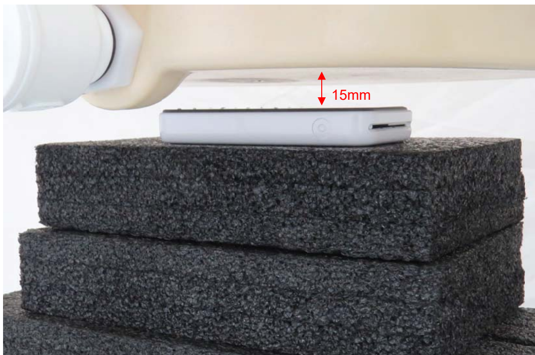
Picture 2: Front Side, the distance from handset to the bottom of the Phantom is 15mm
