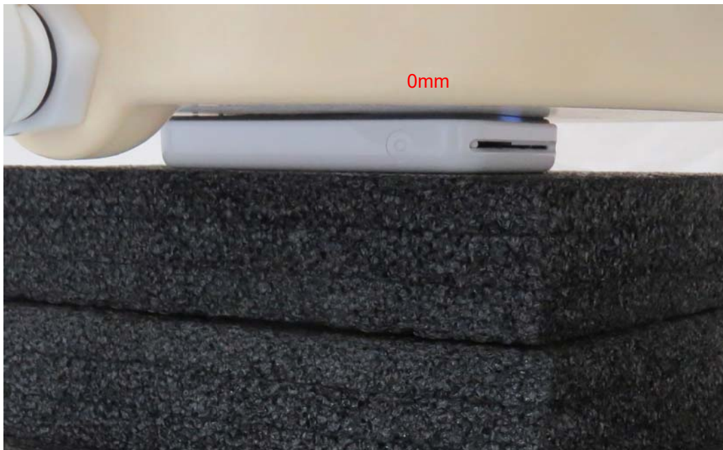
Picture 4: Front Side, the distance from handset to the bottom of the Phantom is 0mm
