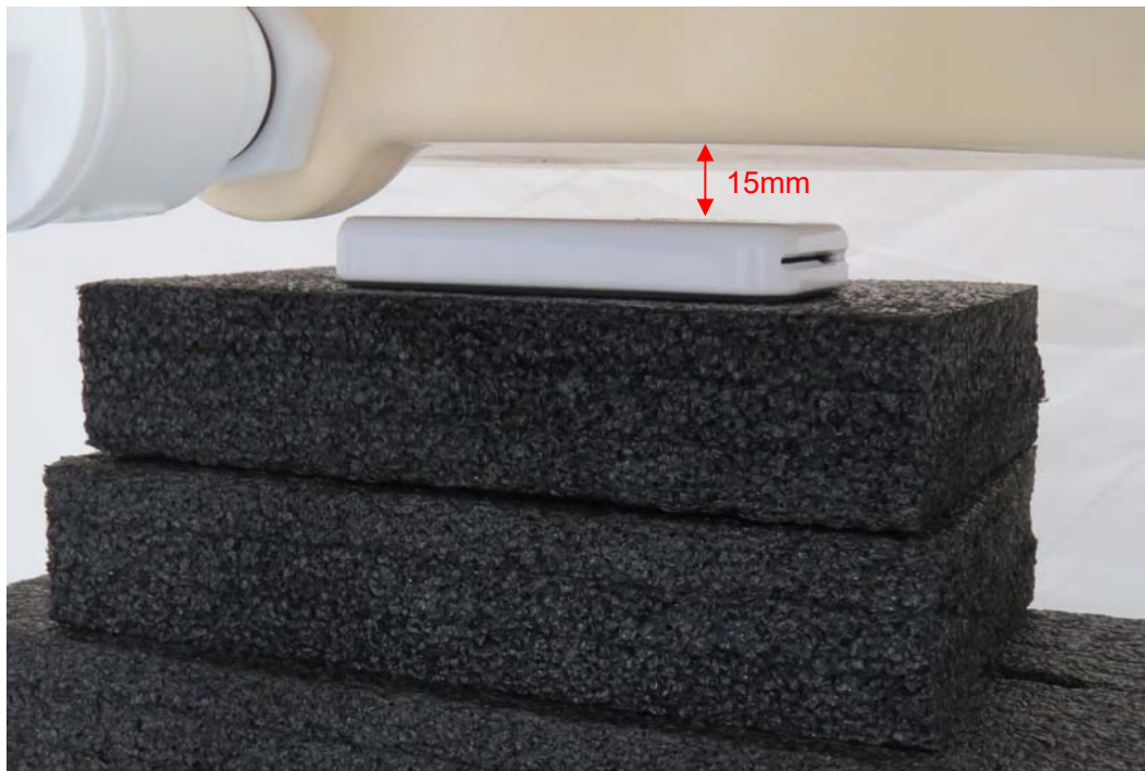
Picture 1: Back Side, the distance from handset to the bottom of the Phantom is 15mm
