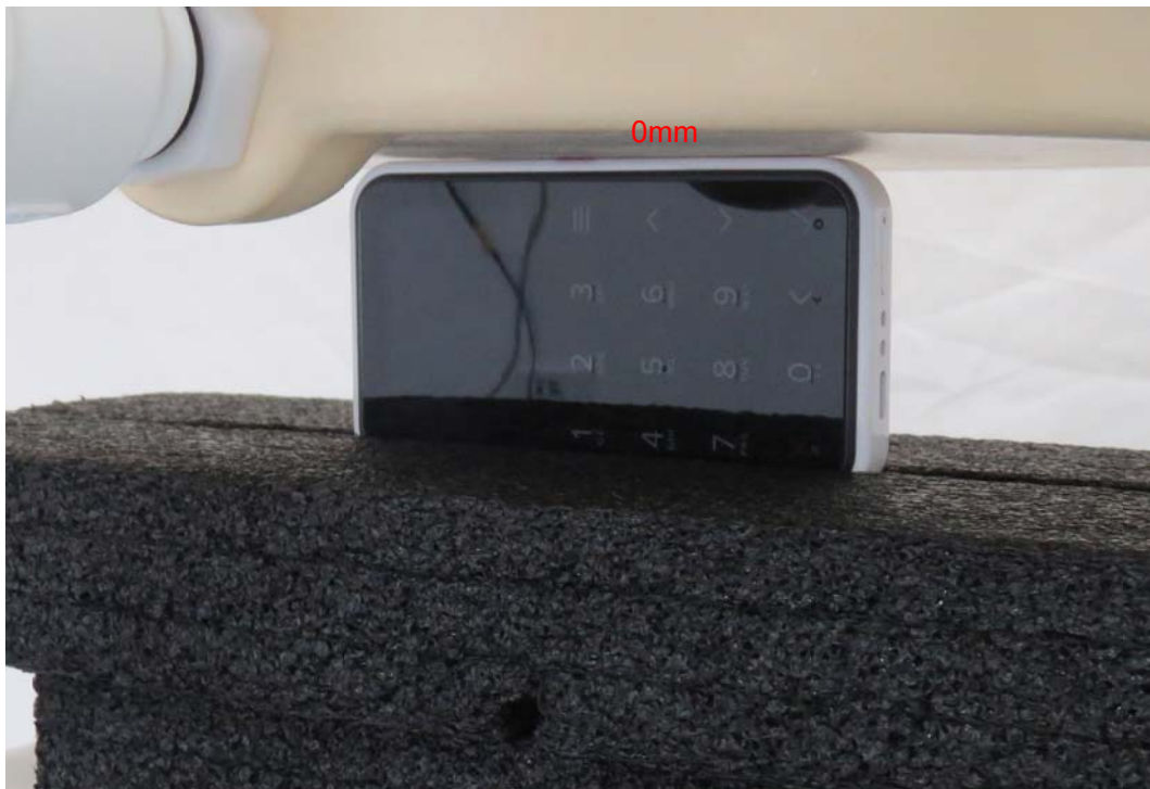
Picture 6: Right Edge, the distance from handset to the bottom of the Phantom is 0mm
